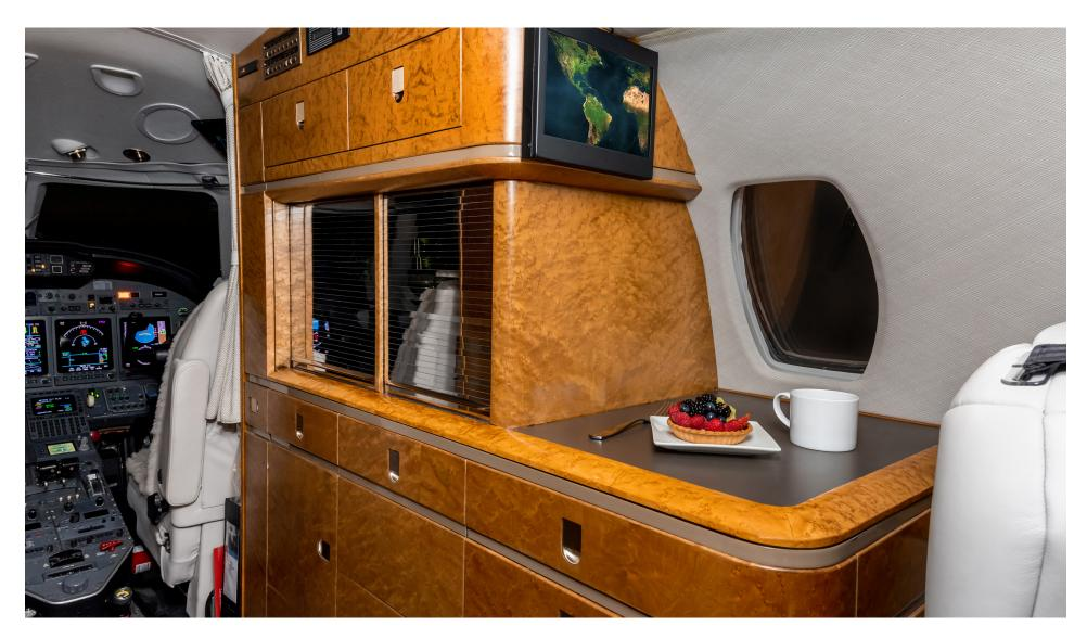
The large galley-bar unit includes miniature liquor storage, gasper cooled beverage can rack, gasper cooled catering drawers, ice drawer with divider, trash container, china, flatware, and crystal storage, and two heated liquid containers. Complete interior refurbishment including refinished wood was accomplished by Southstar Aircraft Interiors in April 2023.
